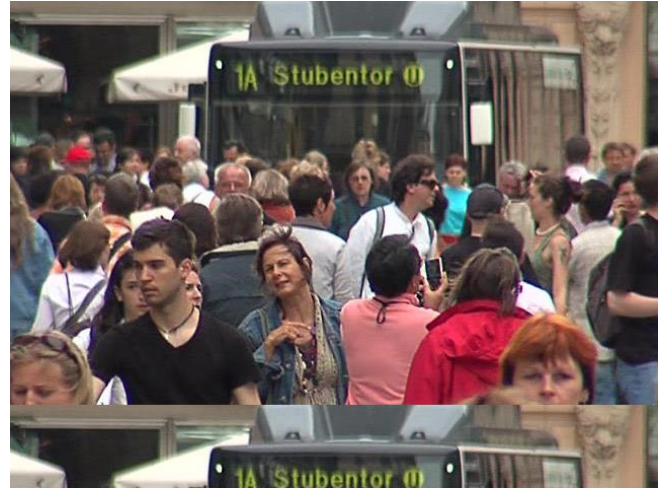
Figure 3 b) Vertical Sync Pulse Loss
