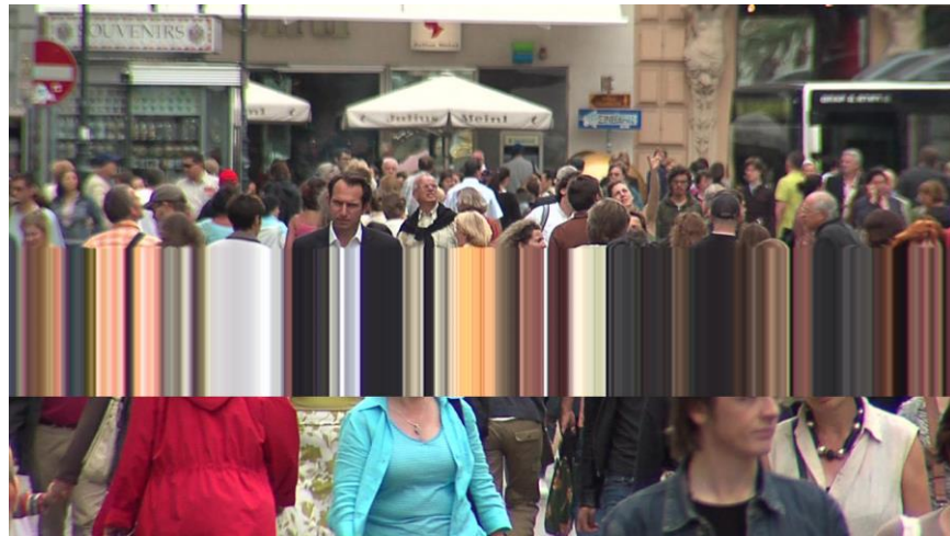
Figure 5. Line Repetition Error
