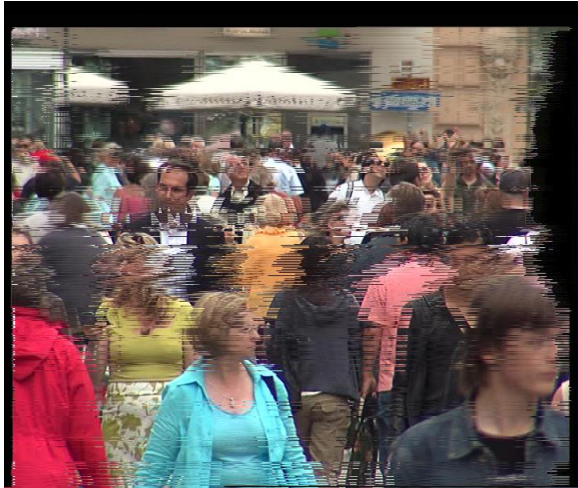
Figure 3 a) Horizontal Sync Pulse Loss
